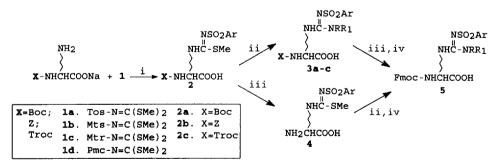
Scheme 1, Reagents and conditions: i. H<sub>2</sub>O/THF; 60 °C; 3-5 h; ii. (A) HNRR<sub>1</sub>/AgNO<sub>3</sub>/MeCN or (B) HgCl<sub>2</sub> in MeCN/DMF, 0-60 °C, 2-12 h; iii. TFA, 0.5 h or HCOOH, 3.5 hs (A=Boc); Zn/AcOH, 1 h(A=Troc); 10%Pd/C in 4.4%HCOOH/MeOH, 10 min (A=Z); iv. Fmoc-OSu/THF/H<sub>2</sub>O/K<sub>2</sub>CO<sub>3</sub>.
